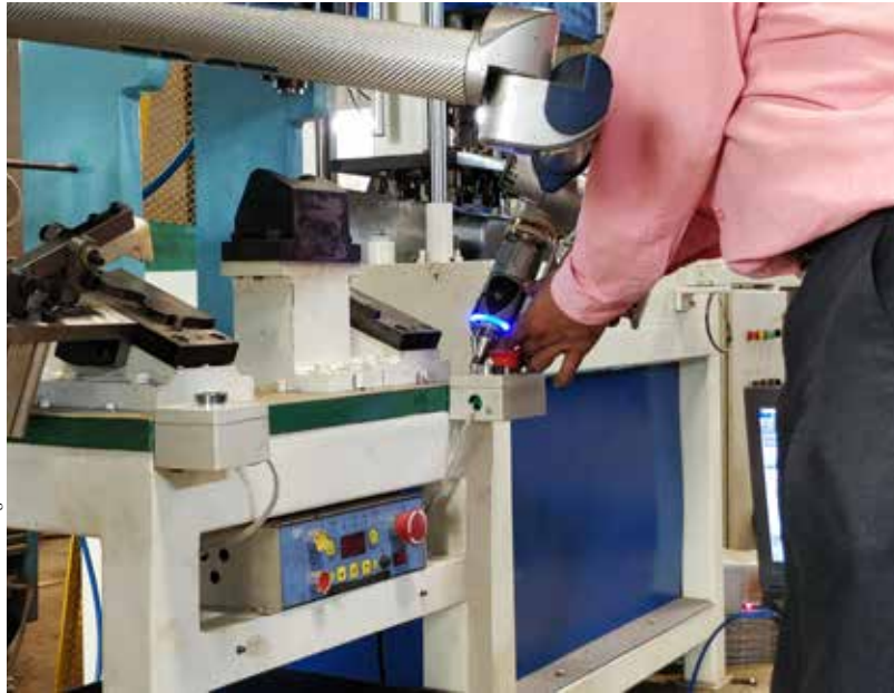
The portable FARO Edge enables inspection anywhere on the shop floor.
