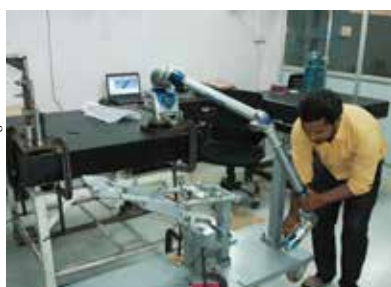
The FARO Edge's infinite rotation allows users to measure anything — even hard-to-reach spots or awkward angles.
