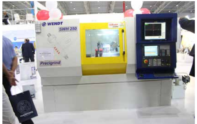
Precigrind, a precision CNC cylindrical grinding machine was unveiled by Ramakant Reddy, Managing Director, LMT FETTE (India) Pvt Ltd. A 3-axis machine with Siemens 828D controls for precision grinding of circular parts, it comes with customised tooling and tailor made diamond/CBN/abrasive wheels for specific applications
