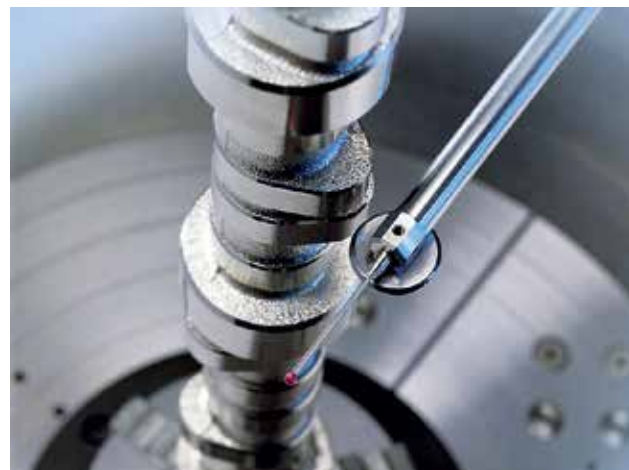
The measuring station measures diameter, gear and form in only one clamping
