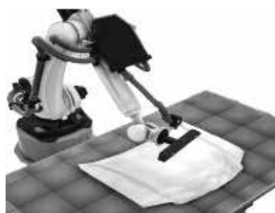
ABIS system surface inspection
